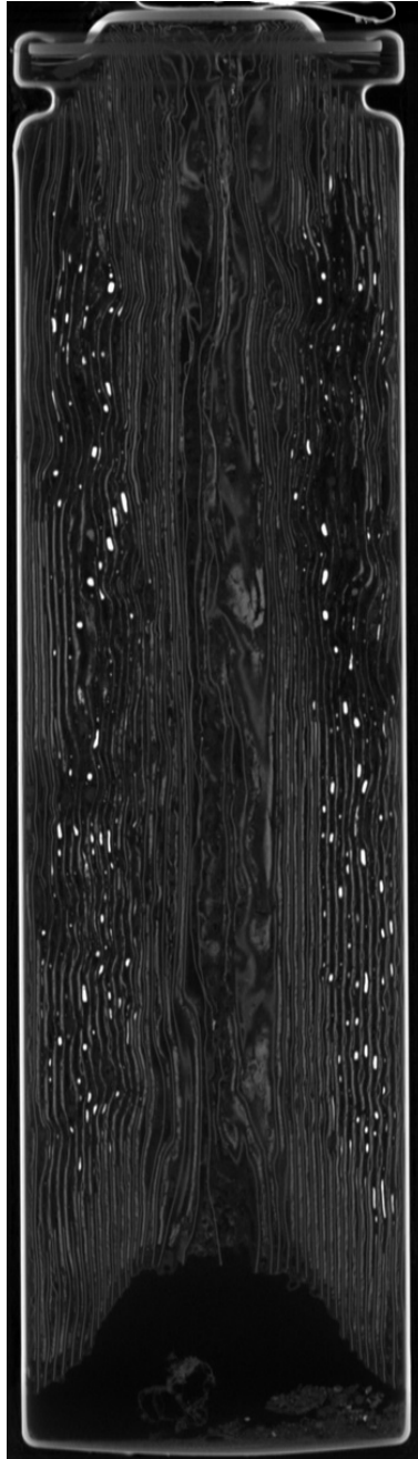
Figure 31. CT scan cross section of an 18650 cell that underwent thermal runaway. Although the electrodes were not ejected, the base to cap pressure differential caused shifting of the electrodes toward the cap.
