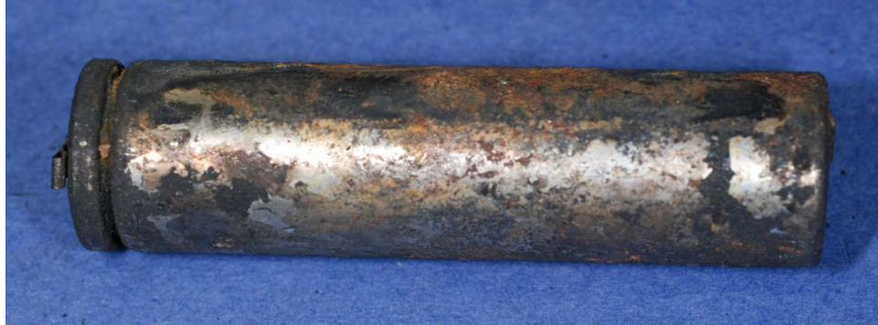
Figure 25. An 18650 cell that has undergone thermal runaway.
