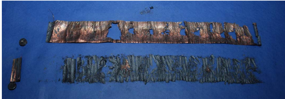
Figure 28. Internal contents of an 18650 cell that underwent thermal runaway: copper current collector (top) and remains of active materials (bottom).
