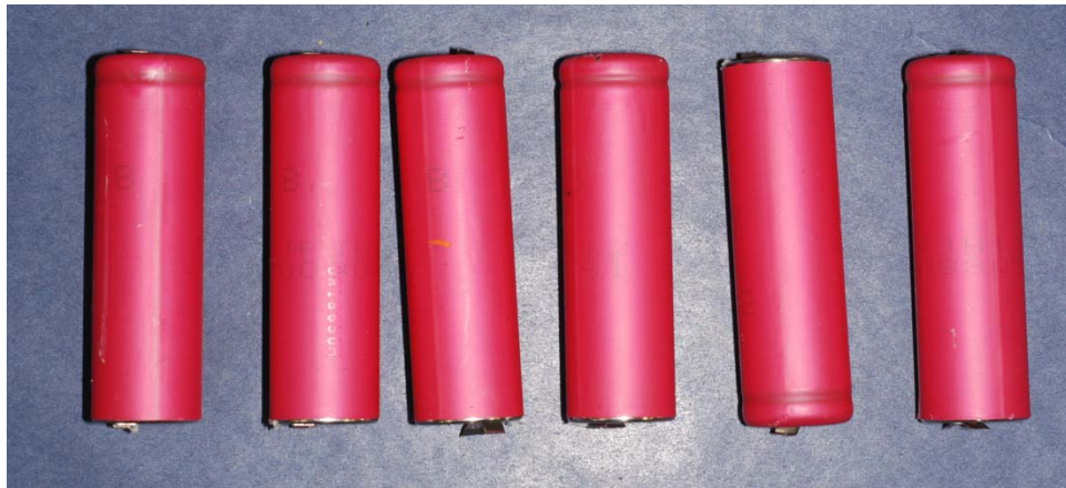
Figure 7. Examples of 18650 cylindrical cells (these are the most common consumer electronics lithium-ion cell form factor).
