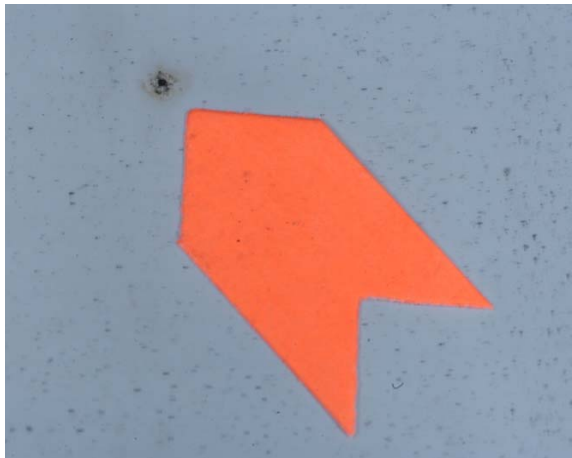
Figure 13. An example of a micro-shorting location on a separator, at the point of shorting, the separator locally melted and shutdown. The micro-short is approximately 1 mm in diameter.
