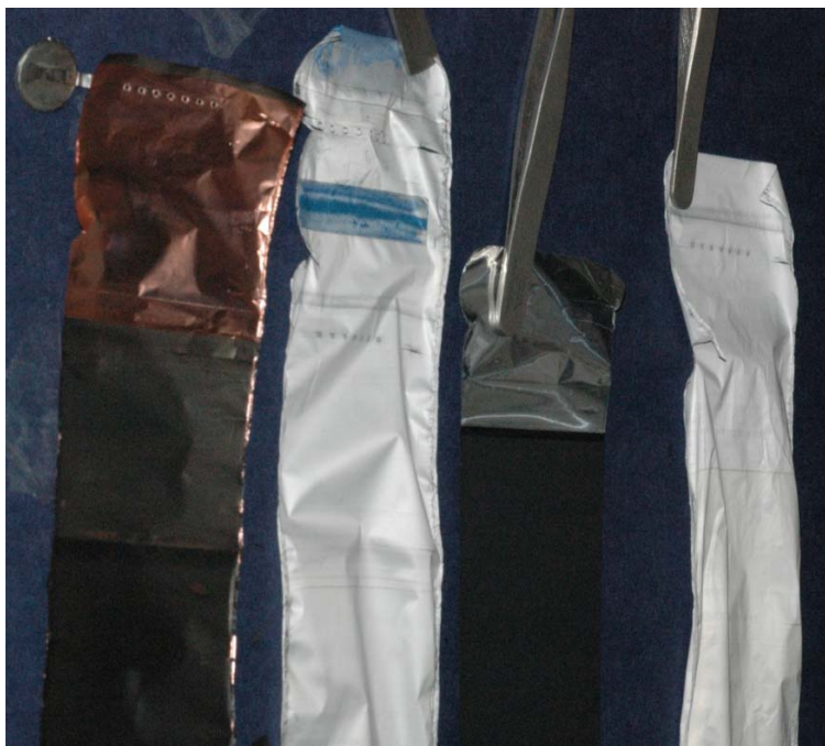
Figure 17. Layers of material from a wound cylindrical cell; left to right: negative electrode (graphite coated onto copper), separator, positive electrode (metal oxide coated onto aluminum), and separator.
