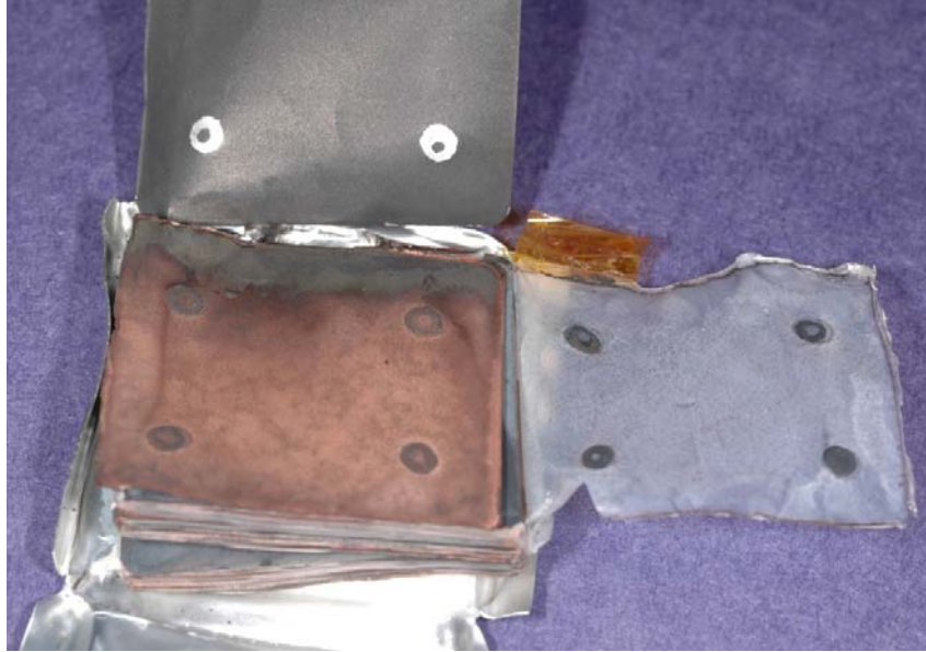
Figure 33. The anode of a repeatedly over-discharged cell coated with copper.
