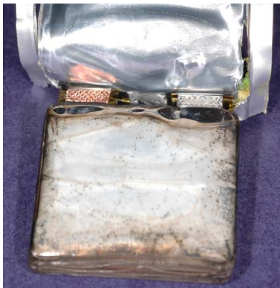
Figure 14. An example of separator melting due to electrical abuse of a cell.
